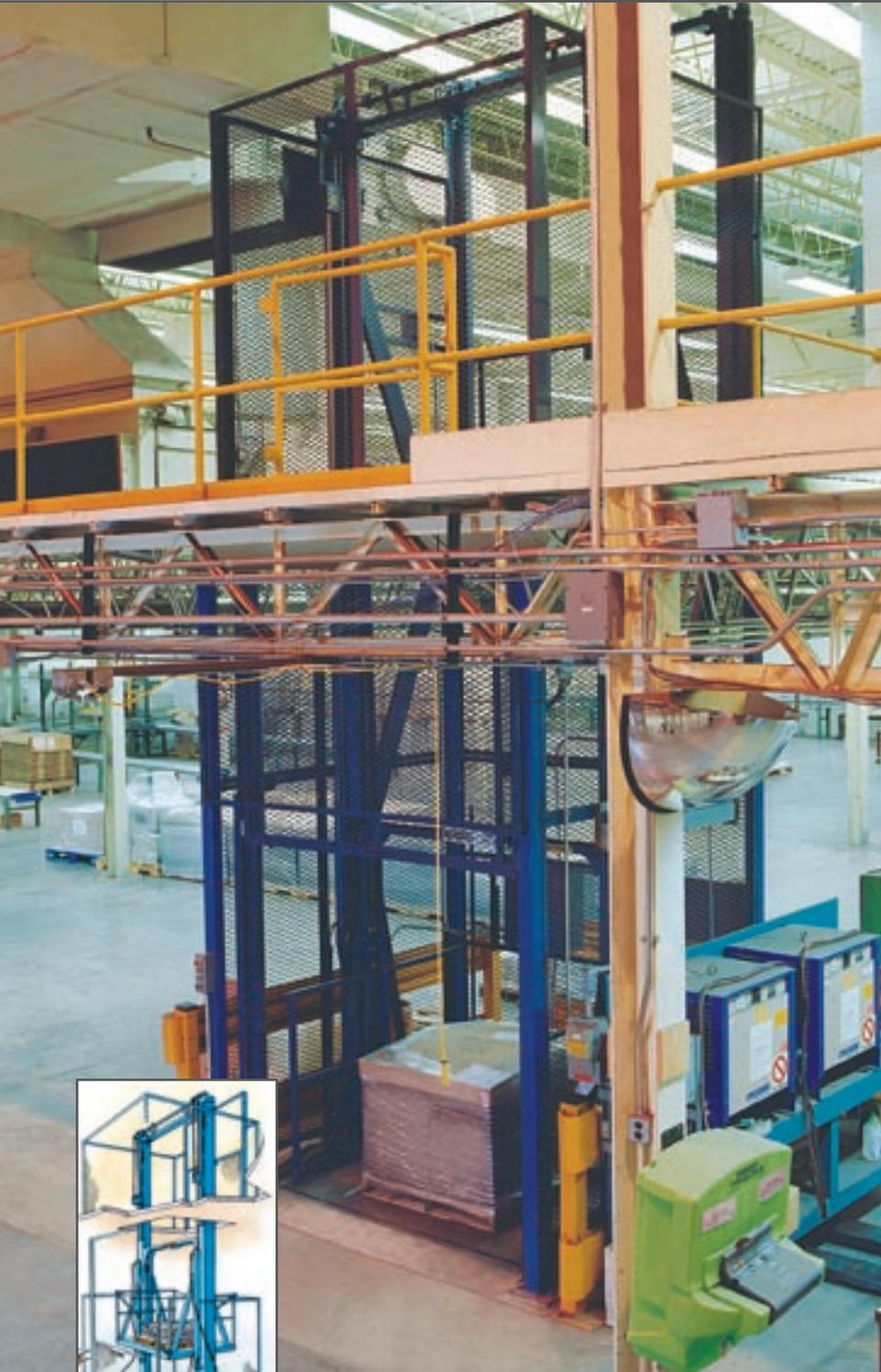
**SERIES 21 LIFT PROVIDES EFFICIENT, SAFE VERTICAL HANDLING FOR LOADS UP TO 8,000 LBS.**
